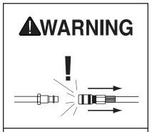
Always disconnect air from nailer whenever servicing! During maintenance, a nailer connected to air may fire accidentally, causing serious personal injury!
